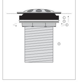
**1.** Clean and remove any loose debris from the drain hole located in the bottom of your sink.
