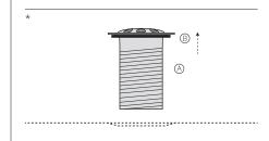
**6.** Apply Thread Seal Tape around the threads of the Tailpiece (F). we recommend wrapping tape securely around the threads at least 4 times.
