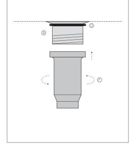
7. Apply Thread Seal Tape around the threads of the Tailpiece (G). we recommend wrapping tape securely around the threads at least 4 times.
